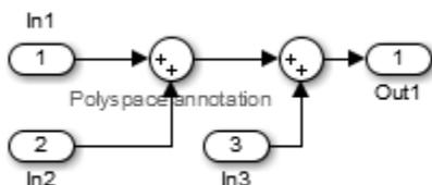
However, the associated generated code adds all three inputs in one line of code.
